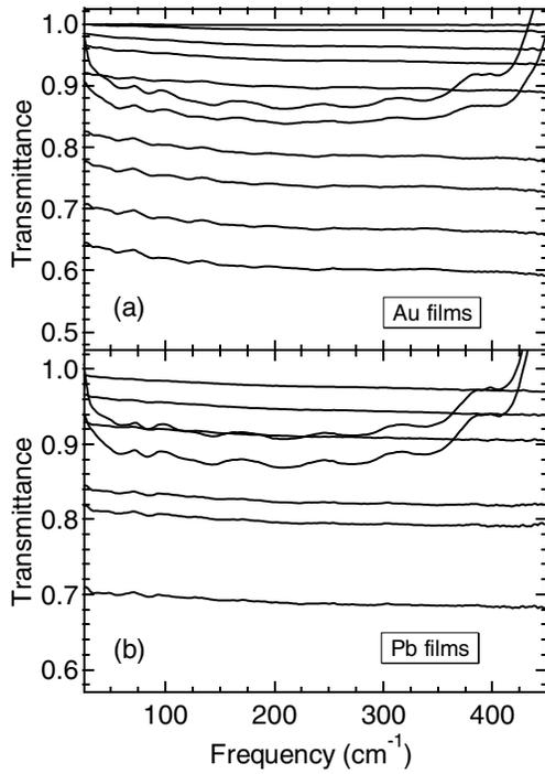
FIG. 1. Far-infrared transmission of UTMF at 10 K. The different curves correspond to different thicknesses. (a) Au films, from top down: 3, 6, 9, 12, 15, 21, 24, 30, and 35 Å. The two curves with anomalous frequency dependence correspond to thicknesses of 18 and 19 Å, respectively. (b) Pb films, from top down: 13, 16, 19, 35, 40, and 51 Å. The two curves with anomalous frequency dependence correspond to thicknesses of 21 and 28 Å, respectively.
