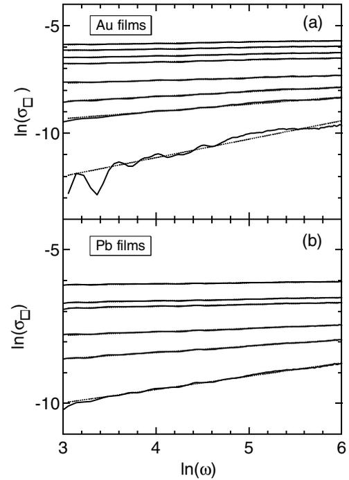
FIG. 3. Sheet conductance of UTMF at 10 K in a log-log plot. The different curves correspond to different thicknesses, and values of the slope  $\beta$  are given in the bracket. (a) Au films, from bottom up: 6 Å(0.9), 9 Å(0.3), 12 Å(0.2), 15 Å(0.1), 21 Å(0.09), 24 Å(0.08), 30 Å(0.07), and 35 Å(0.07); (b) Pb films, from bottom up: 13 Å(0.4), 16 Å(0.2), 19 Å(0.1), 35 Å(0.06), 40 Å(0.06), 51 Å(0.04).
