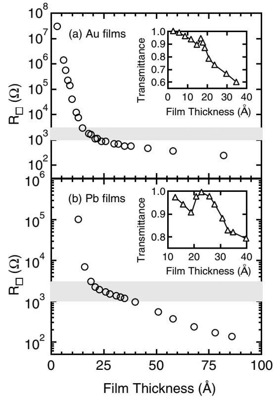
FIG. 2. The thickness dependence of the sheet resistance,  $R_{\square}$ , of UTMF. (a) Au films; (b) Pb films. The shaded section corresponds the region where the anomalous transmission occurs. Insets: The thickness dependence of the transmittance at a fixed frequency of  $425 \text{ cm}^{-1}$ .
