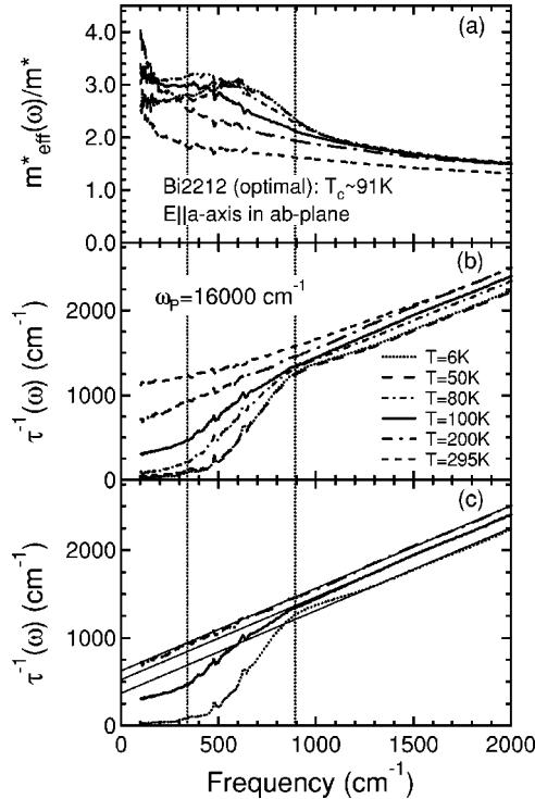
FIG. 2. The analysis of the  $ab$ -plane optical data of an OP Bi2212 single crystal with the  $E \parallel a$  from 100 to 2000  $\text{cm}^{-1}$ . (a) The temperature-dependent mass ratio, (b) the temperature-dependent  $\tau^{-1}(\omega)$ , and (c)  $\tau^{-1}(\omega)$  is analyzed at 6, 100, and 200 K.
