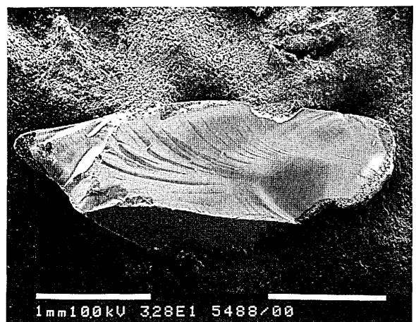
Fig. 5. Irregular piece broken from a crystal of SrTiO<sub>3</sub> used to measure the spectra in Fig. 6.
