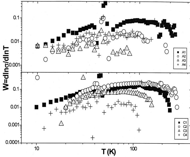
FIG. 3. Log-log plots of the activation energy  $W$  against temperature for PANi-AMPSA (top) and PANi-CSA (bottom). Both sets of curves show a prevailing positive slope, even though the PANi-AMPSA curves are considerably more erratic.
