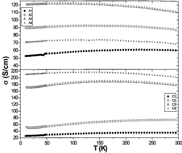
FIG. 2. Temperature dependent dc conductivity graphs for PANi-AMPSA (top) and PANi-CSA (bottom) samples. The positive TCR is more pronounced for the most conducting samples A3 and C4.
