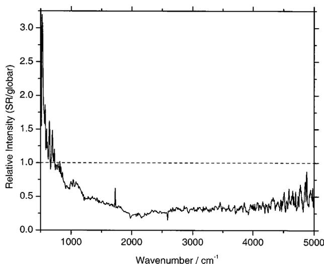
FIG. 3. Ratio of SR PA spectrum of carbon-filled rubber to the corresponding Globar<sup>®</sup> spectrum, obtained with an aperture of 2 mm. The dashed line at 1.0 is drawn as an aid to the reader.
