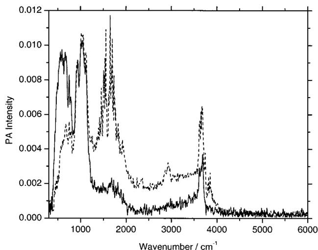
FIG. 2. Mid-infrared PA spectra of common clay, obtained with a 1 mm beam. Solid line, synchrotron radiation (SR); dashed line, Globar<sup>®</sup>.
