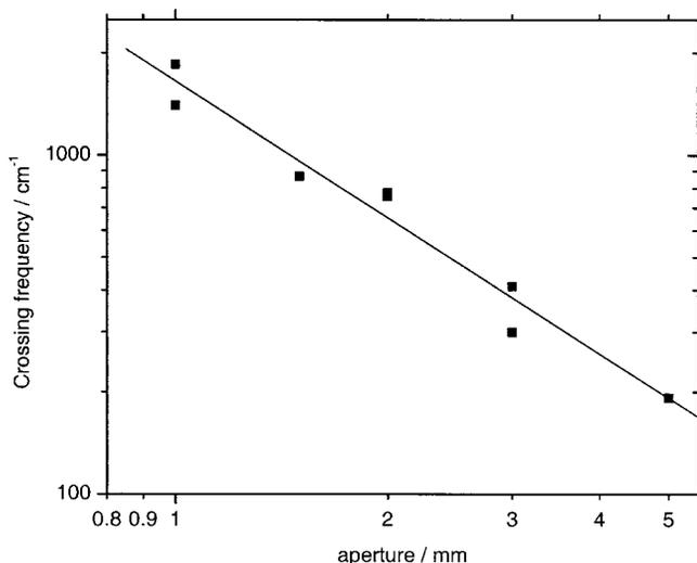
FIG. 5. Dependence of crossing frequency on aperture size. The crossing frequency is the wave number at which SR PA intensity equals Global<sup>®</sup> PA intensity. The solid line is a least-squares fit to the data.
