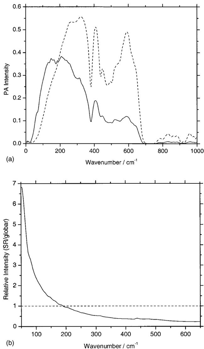
FIG. 1. (a) Far-infrared PA spectra of glassy carbon, obtained with two different sources of infrared radiation. Solid line, synchrotron radiation (SR); dashed line, Global<sup>®</sup>. (b) Ratio of the SR spectrum in (a) to the Global<sup>®</sup> spectrum. The dashed line at 1.0 is drawn as an aid to the reader.
