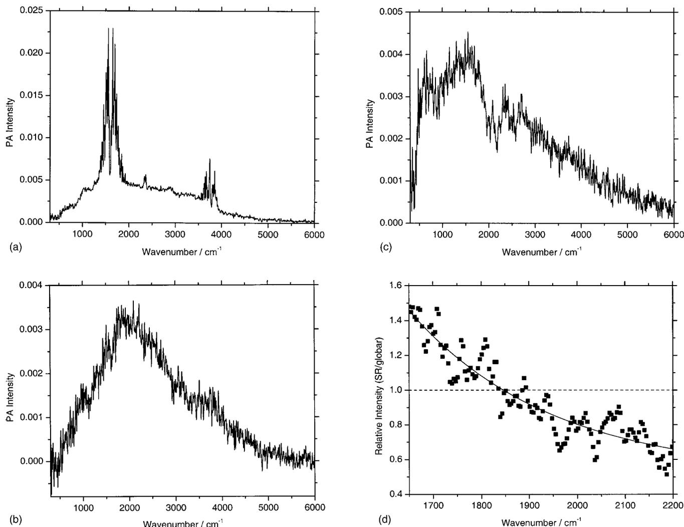
FIG. 4. Mid-infrared PA spectra of carbon-filled rubber, obtained with a 1 mm beam: (a) Globar<sup>®</sup> spectrum, (b) Globar<sup>®</sup> spectrum after subtraction of spectrum due to water vapor, (c) SR spectrum, and (d) ratio of spectrum in (c) to that in (b). The solid line in (d) is an experimental fit to the data; the dashed line at 1.0 intersects this curve at the frequency where SR and Globar<sup>®</sup> PA intensities are equal.
