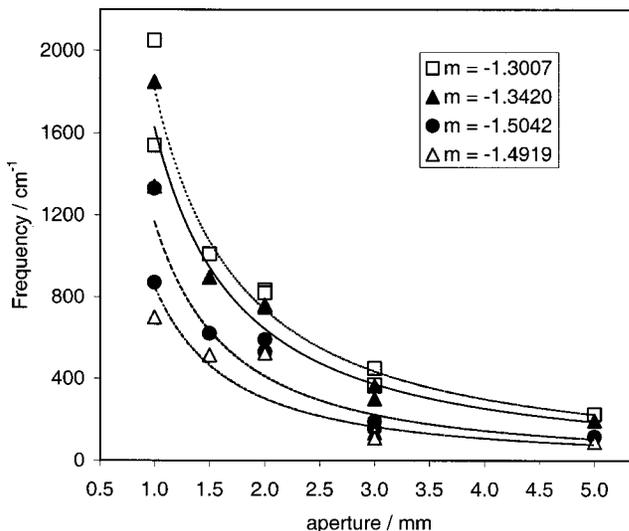
FIG. 6. Variation of frequency with aperture size for selected SR/Global<sup>®</sup> intensity ratios. The curves represent power-law ( $\nu \propto x^m$ ) fits to the experimental points (see legend). Ratios represented in this graph are 0.8 (open squares, dotted line), 1.0 (filled triangles, solid line), 2.0 (filled circles, dashed line), and 2.8 (open triangles, dash-dotted line).
